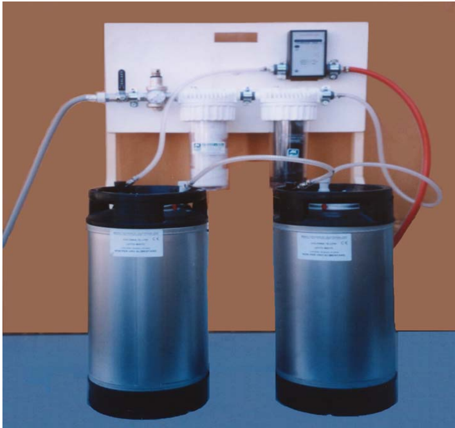
LED bargraph conductivity meter
